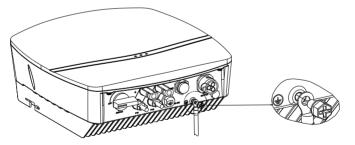
Fig. 5.5 Inverter ground protection
