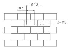
Figure 4.7 Drill holes' dimensions of R5-3K/3.6K/4K/5K/6K/7K/8K-S2,
