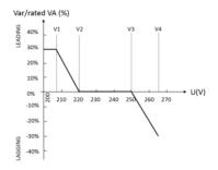
Figure 6.11 Curve for a Volt-Var control mode (AS4777 Series)
