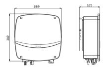
Figure 3.2 Dimensions of R5-0.7K/1K/1.5K/2K/2.5K/3K-S1
