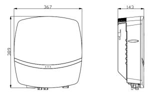
Figure 3.4 Dimensions of R5-3K/3.6K/4K/5K/6K-S2
