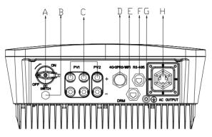
Figure 5.4 Electrical interface of R5-7K/8K-S2
