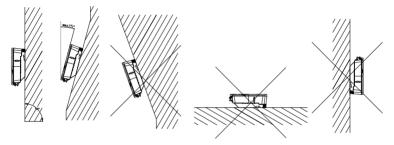
Figure 4.1 Mounting method
