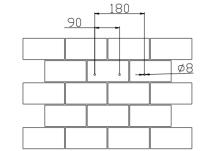
Figure 4.6 Drill holes' dimensions of R5-0.7K/1K/1.5K/2K/2.5K/3K-S1
