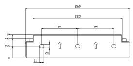
Figure 4.3 Dimensions of rear panel of R5-0.7K/1K/1.5K/2K/2.5K/3K-S1 R5-0.7K/1K/1.5K/2K/2.5K/3K-S1-15
