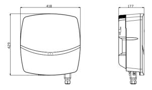
Figure 3.5 Dimensions of R5-7K/8K-S2 R5-7K/8K-S2-15
