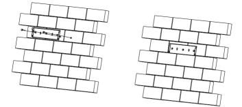
Figure 4.8 Mount the rear panel of R5-0.7K-3K-S1/ R5-0.7K-3K-S1-15
