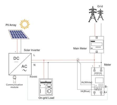
Figure 6.13 Export limitation system schematic
