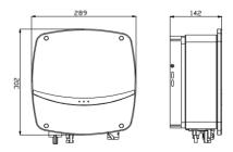
Figure 3.3 Dimensions of R5-0.7K/1K/1.5K/2K/2.5K/3K-S1-15
